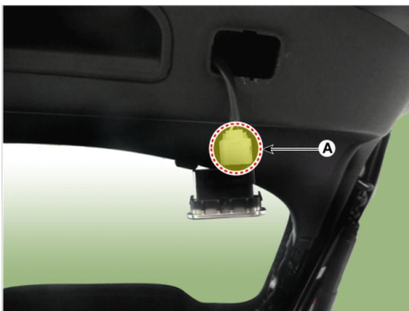
6. Remove the tailgate trim (A) after loosening the mounting screws.
