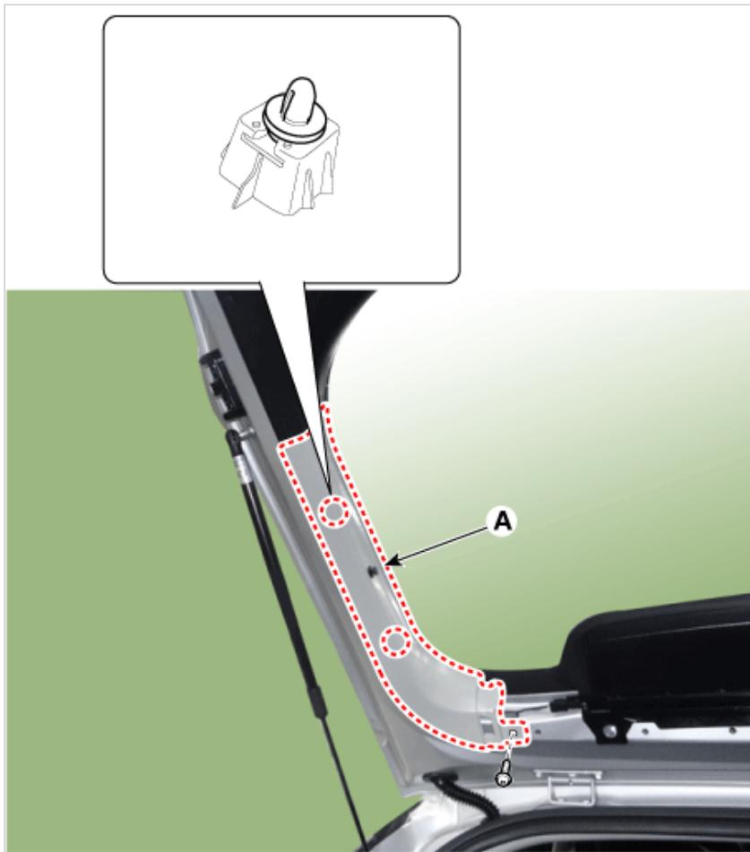
3. Remove the tailgate inside full handle cap (A) by using a remover.
