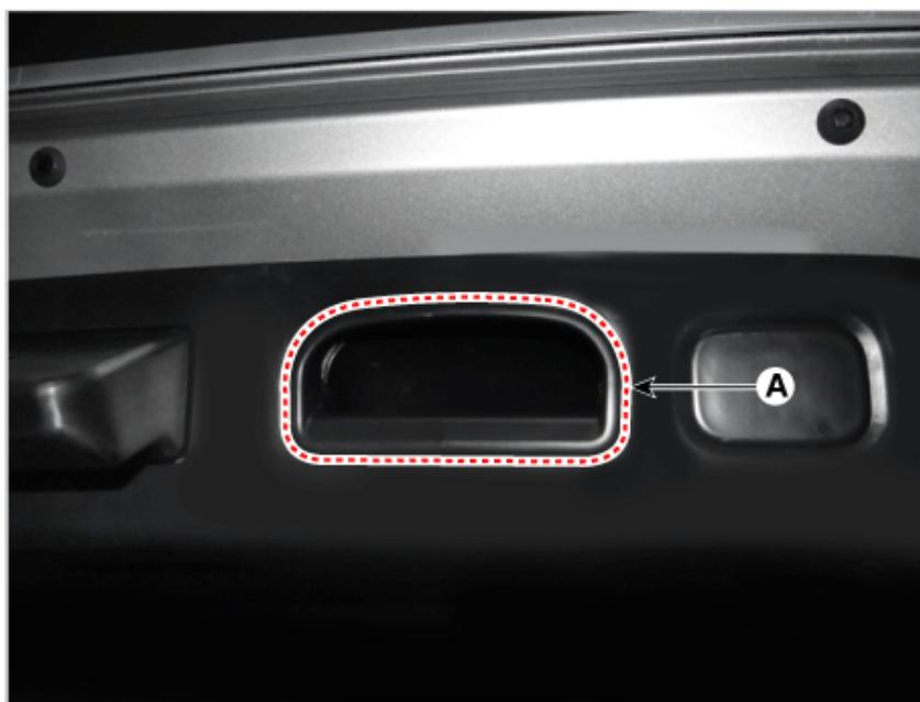
4. Separate the smart tailgate inner switch (A).
